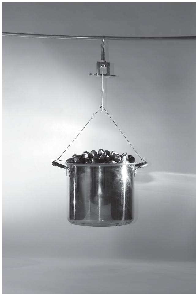
Figure 1. A pot full of mussels being held up by aluminum substrates bonded together in shear with poly[(3,4-dihydroxystyrene)- co -styrene].
